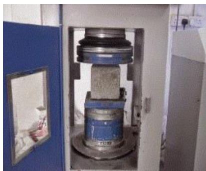
Fig.3.Compressive Strength test on Cube
